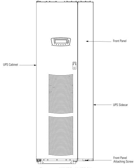
Figure 2-1. 80 kVA UPS with UPS Sidecar
